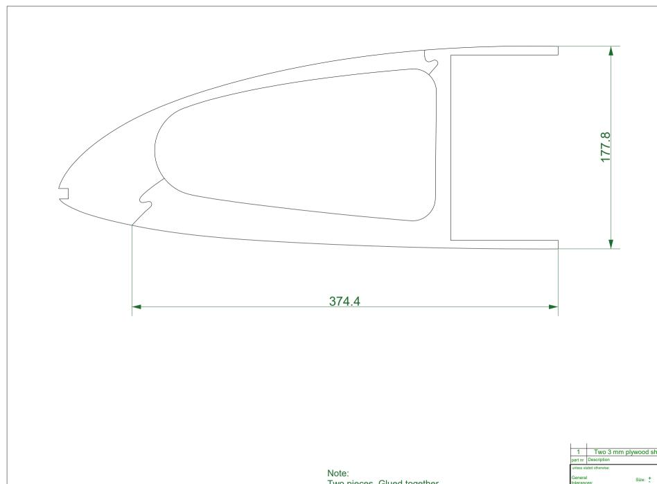
Two pieces. Glued together after fuel tank is installed.
