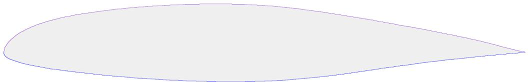
Profile selection was based mainly on reference <http://www.n56ml.com/as504x/default.htm> on design of new airfoil for KR-2S wing by Ashok Gopalarathnam. The AS5045 airfoil selected for KR-2S was little bit better than NLF(1)-0115, but due to sharper leading edge the more round NLF(1)-0115 was selected for this aircraft.
