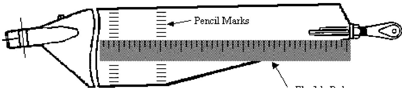
Bottom View of Forward Lift Strut
