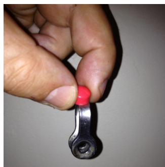
Shackle fails the test by being easily suspended by the magnet
